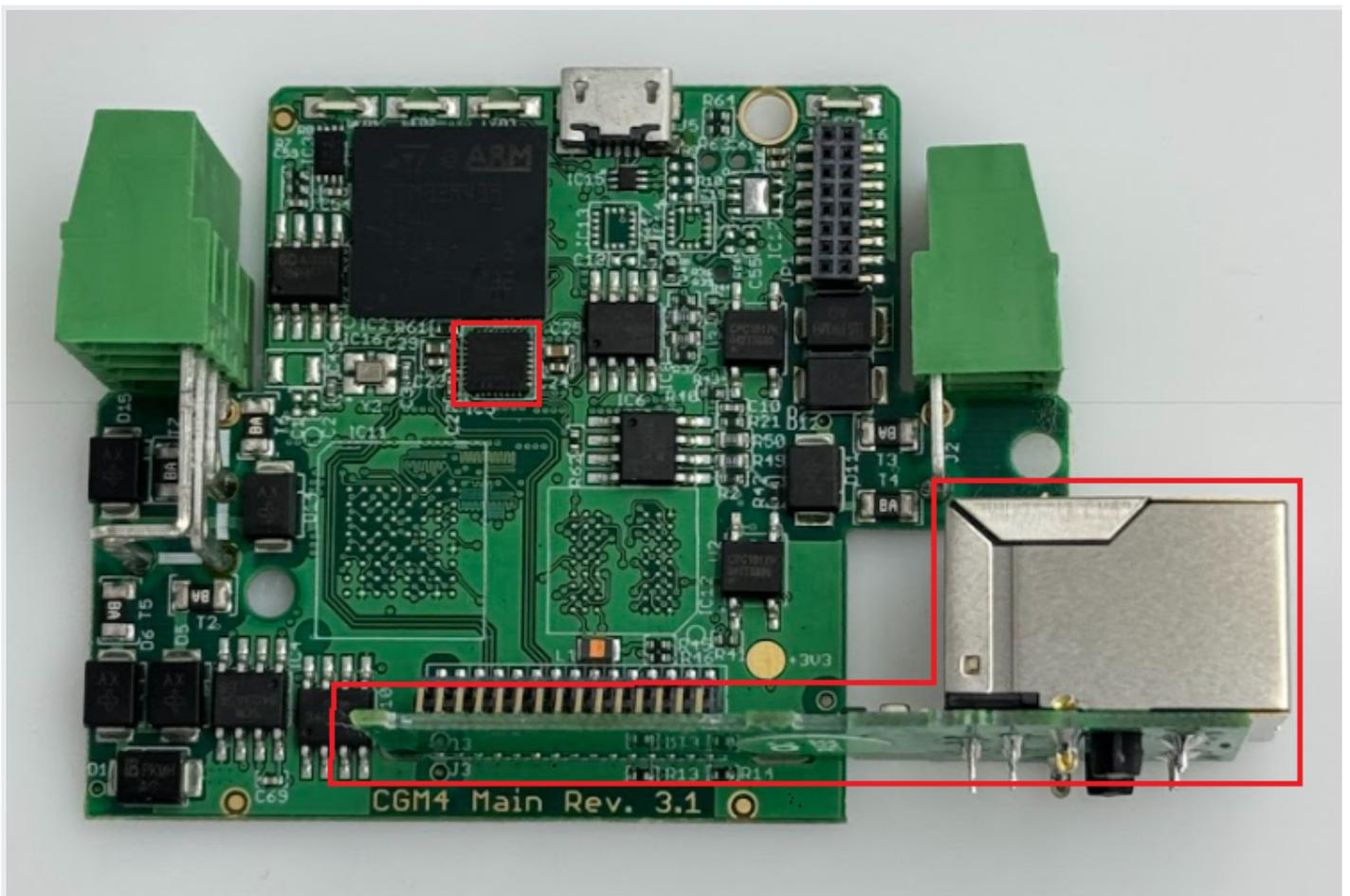
This example allows you to check the Gateway's IP address. Connect the device via USB/UART converter and choose correct COM/ttyUSB port. Remember to connect the IoT Gateway to the network using an Ethernet cable. Type in terminal "ipconfig". If your network connection works
