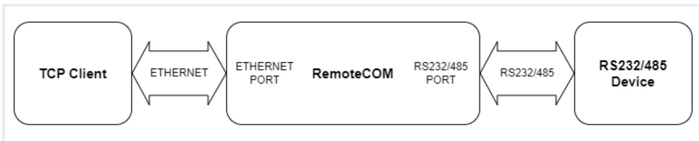
Then, it is necessary to configure the RemoteCOM's ports. It can be done, for example, via the device's web page. Ports' configuration can be also done via the Telnet, serial or service console. Set the "**TCP Socket**" option in the "Service" field on the "Port" page. Check also if the port number is set correctly in the "Port" field. Set desired options of the RS232/485 connection ("Baud Rate", "Data Bits", "Parity", "Stop Bits" - these options should be the same as in the RS232/485 device).
