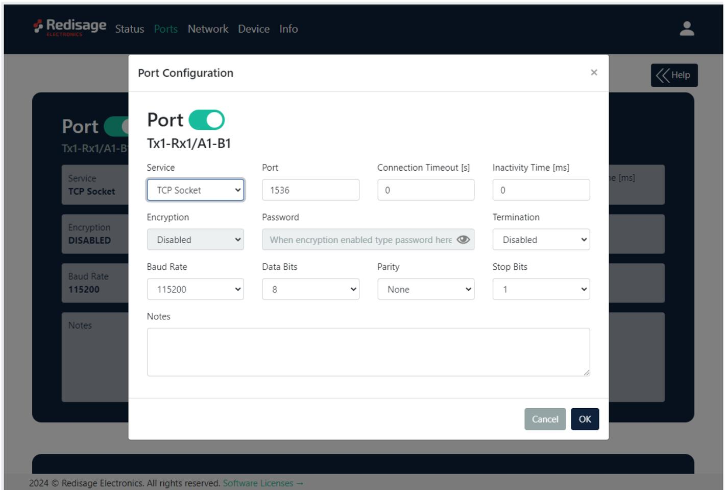
Now, the device should be ready to work. Once the TCP Client creates a TCP socket, the bidirectional communication should be available.
