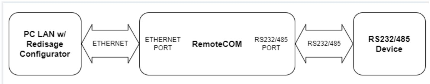
Then, it is necessary to configure the RemoteCOM's ports. It can be done, for example, via the device's web page. Ports' configuration can be also done via Telnet, serial or service console. Set the "RemoteCOM" option in the "Service" field on the "Port" page. Check also if the port number is set correctly in the "Port" field. Additionally, encryption can be set to increase the security (it will also require to set up a password).
