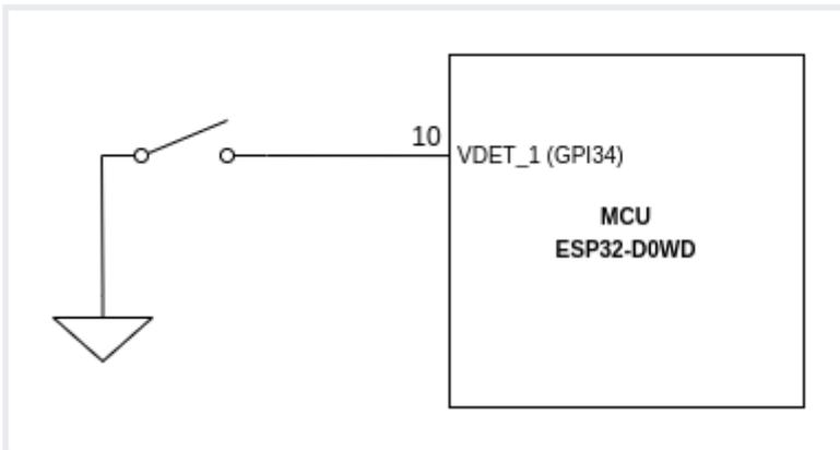
The Open IoT Gateway P01 variant contains a tactile switch. The PCB has hardware pull-up designed into it so debouncing effect is eliminated.
