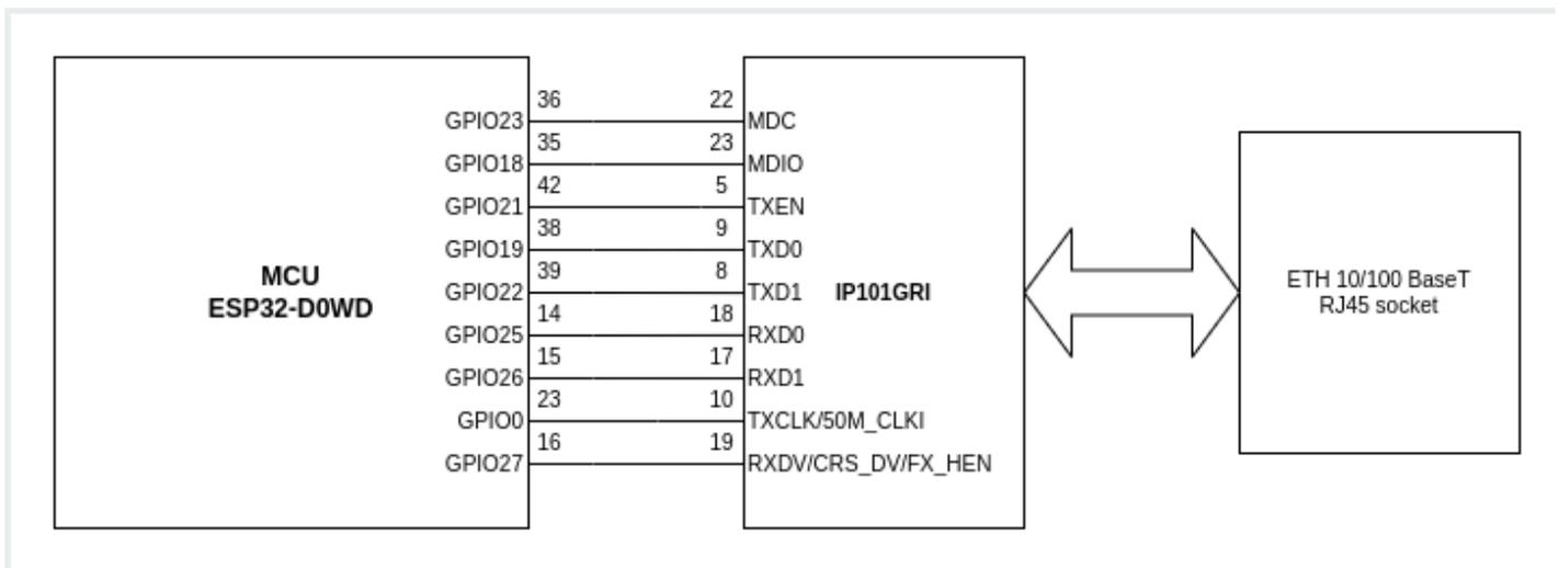
The Ethernet interface is provided by the IP101G physical layer. There is also an external board with RJ25 socket which ensures wired connection to the network.
