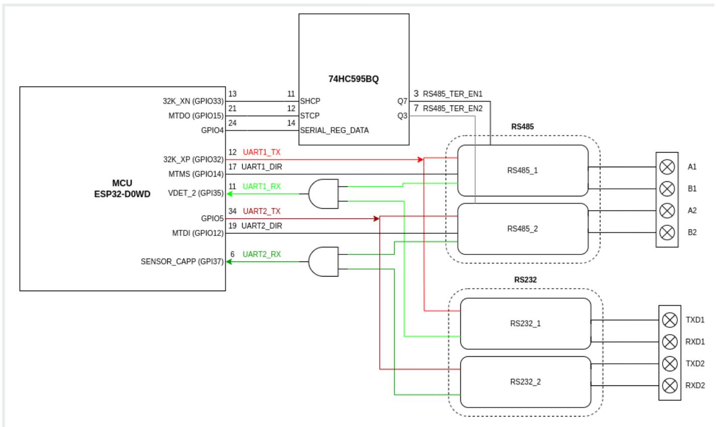
The gateway is equipped with 2 transceivers MAX481 that handle transmission in RS485 standard on each channel independently. Similar to RGB, each channel can be enabled by SIPO shift register 74HC595BQ.
