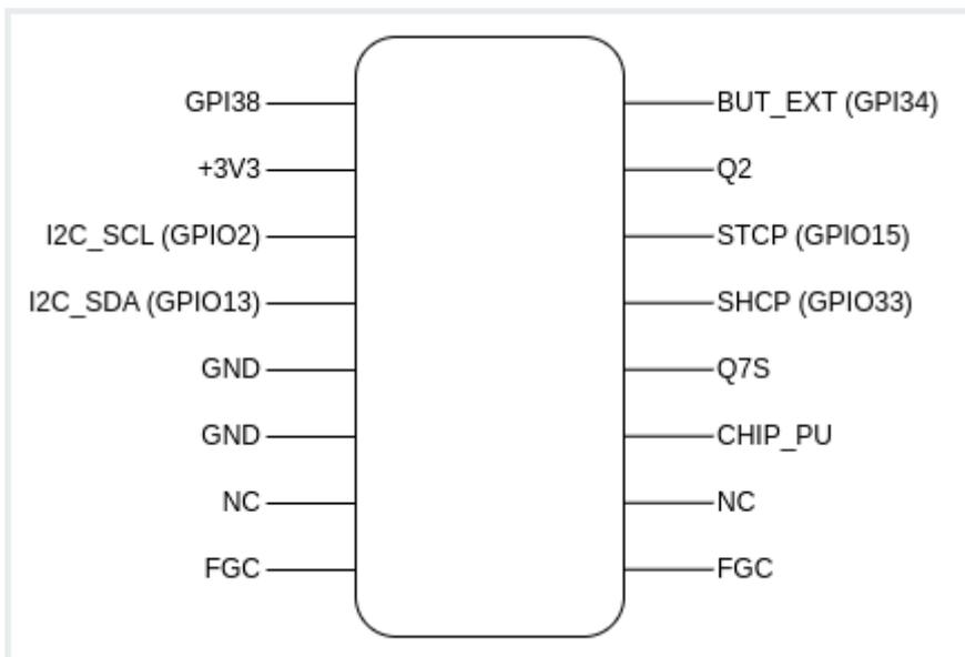
The female goldpin connector allows easy access to different signals. It might be useful during analysis of the board.
