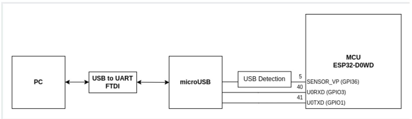
MicroUSB ensures access straight to UART interface (UART0). The Open IoT Gateway does not have inbuilt FTDI converter so an external USB to UART FTDI converter is needed to run a serial port monitor on a PC.
