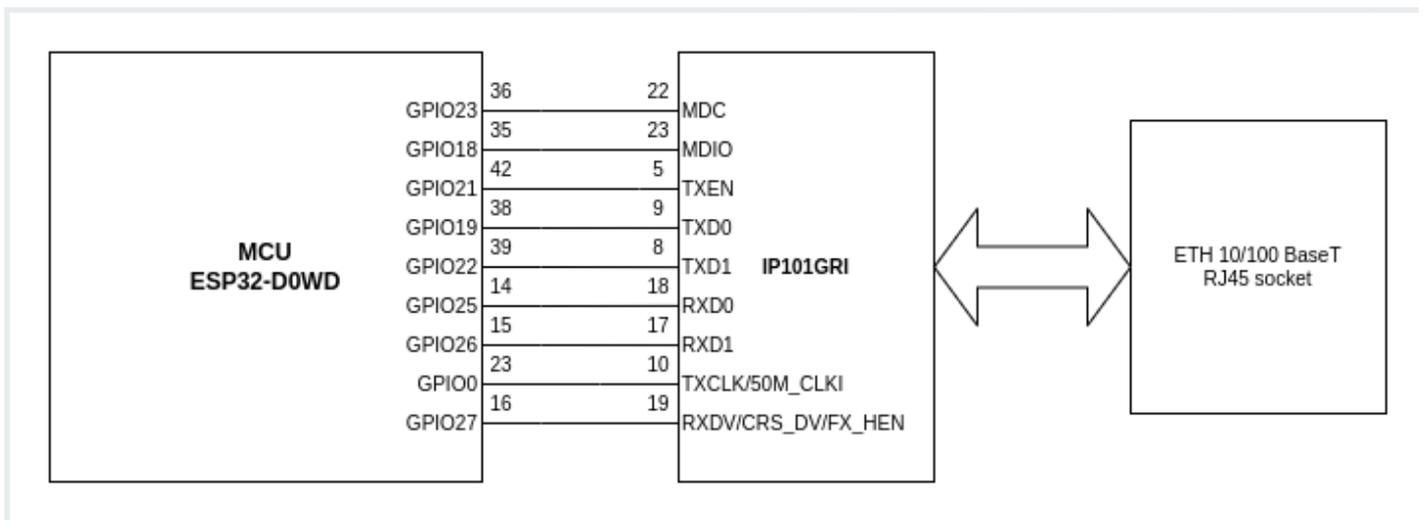
The Ethernet interface is provided by the IP101G physical layer. There is also an external board with RJ45 socket which ensures wired connection to the network.
