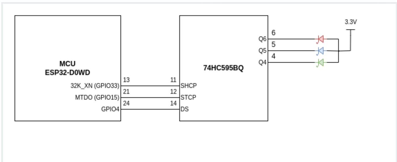
RGB LED is controlled by SIPO shift register 74HC595BQ.
